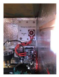
**Emergency panel switch connects house bank to the starter battery.** This is in the event the start bank is dead. The switch is on the port side back wall of the engine compartment. Once the engine has started, turn the switch back to the off position and proceed with motoring.
