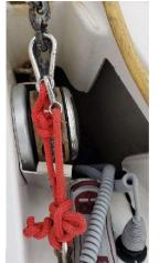
The **anchor tension line (snubber)** is red and used to keep the primary anchor chain taut and remove stress from the windlass when underway. **Do NOT use when anchored**.
