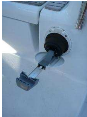
Manual bilge pump lever unfolded and extended
