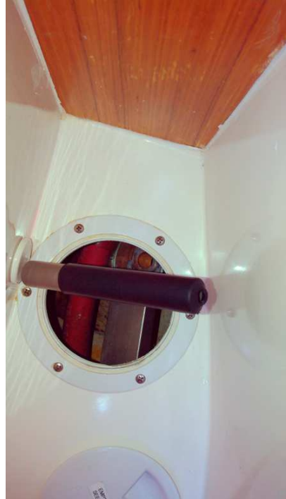
Drop C-channel over valve handle so that walls engage with handle
