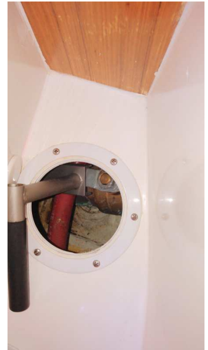
Turn handle 90 degrees clockwise with C-channel engaged on valve handle
