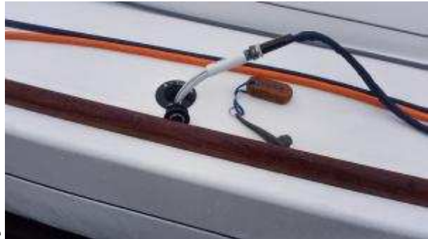
Hose stub allows easy filling of water tanks
