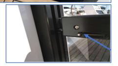
**Salon Lighting Controller and other Cabin Light Switches** – The salon lights are operated by an electronic controller <u>located on the inboard end of the galley "L" cabinet</u>. After turning on the "LIGHTS" breaker on the DC Panel at the navigation station, a quick press on the Power Button followed by a press the S1 button will turn on all lights at once (except galley lights). Pressing the S1 button a second time will turn them off. Press S2 to turn on the two galley lights.
