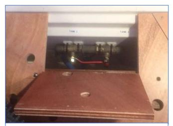
Water Tank Valves under starboard side of V-berth cushion.
