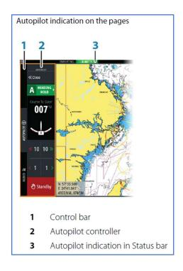
Alternatively, you can select the Autopilot on the far left edge of the GPS window to pull up the Autopilot Control Bar on the left side of the screen. It has the same controls as the controller, but makes the autopilot controls more accessible if you are keeping watch from the Port side of the boat.
