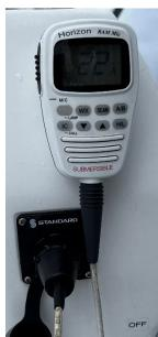
**Turning On and Off the radio** – Flip on the VHF RADIO breaker switch on the DC panel. The power switch on the radio is the Volume knob (upper right gray knob) – turn clockwise.
