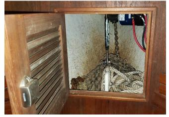
flashlight through the door in the v-berth) to make sure the chain is not stacking up on the incline panel or going over onto the wrong side of the anchor.
