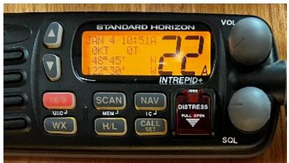
DSC alarm it sounds an alarm on all boats in the area. Press the up/down arrow to view the nature of the alert. To silence this alarm, press any key on the radio. **Note:** do not simply silence an alarm without understanding the nature of the emergency.
