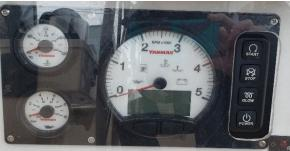
operating correctly. (NEVER turn off the Power with the engine running as it may blow the diodes on the alternator and it will cease to chart the batteries; push the Stop button first.)
