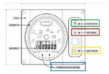
Stopping the Engine: Do not hit the ON/OFF power switch while the engine is running. It's like turning off a traditional engine key while the engine is running which can blow the alternator.
