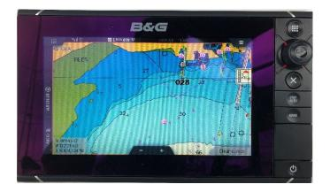
**Depth Sounder**: The B&G unit's measurement is set in feet. There is no "Keel Offset". That is; the transducer is set to where it is. The bottom of the hull. With a draft of 7 feet, If you're reading 5 feet of depth, you're likely aground.
