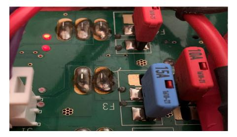
Note: The above picture is not necessarily the exact fuse you will reset. Look at all resettable fuses and push in the small tab as necessary.
