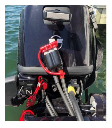
CAP BATTERY CABLE WHEN NOT USING BATTERY
