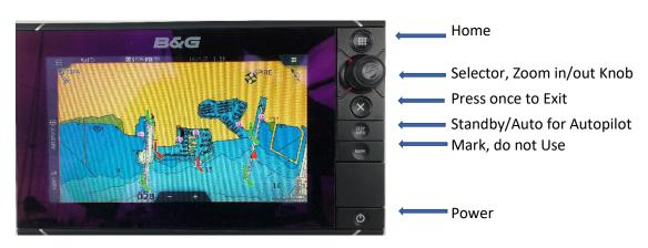
**Finding Home Page/Main Menu:** After turning on the Power Key, hit the Home Key to find the Chart Plotter, Radar, and Tides functions. We recommend that you only use these three functions. The Autopilot is much easier to manage at the small control at the starboard helm. Guests are asked not to set waypoints and routes because the "drift" impact of Pac NW currents require constant attention.
